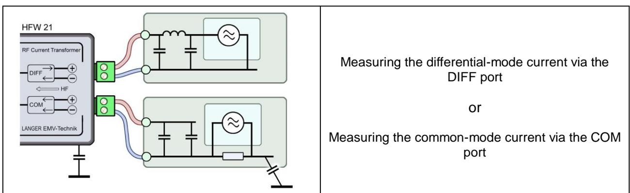
Measuring the differential-mode current via the DIFF port
