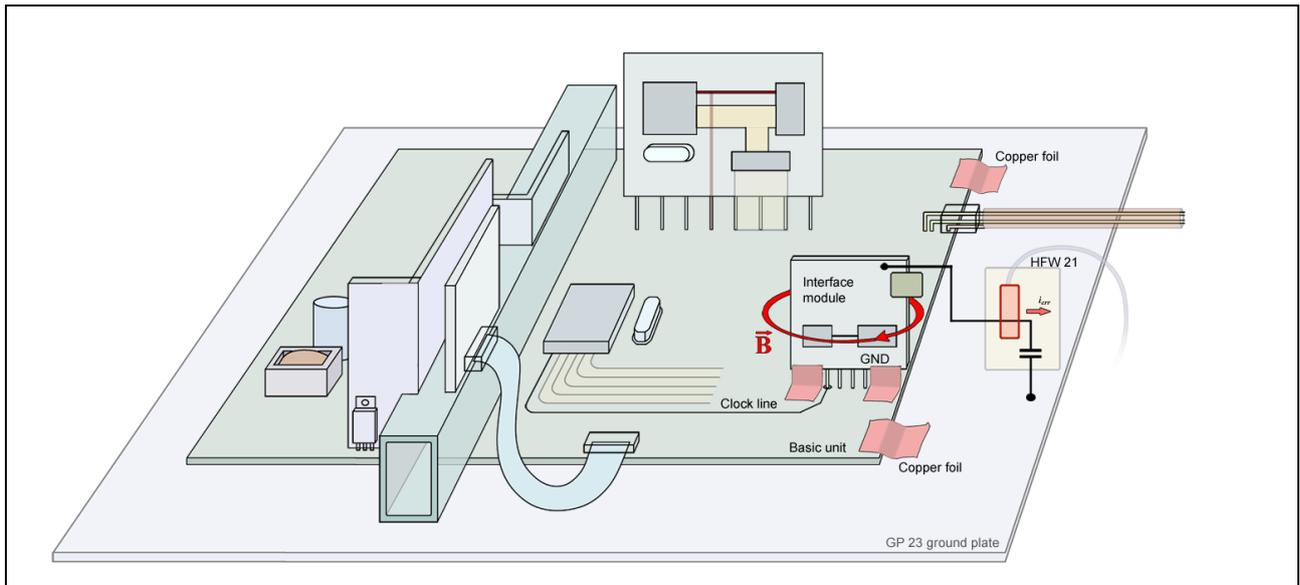
**Figure 29** Evaluation of the modifications with the HFW 21
