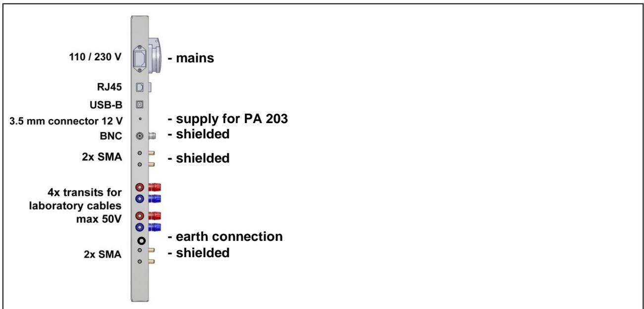
Figure 3 Connections/transits of GP 23 Ground Plate
