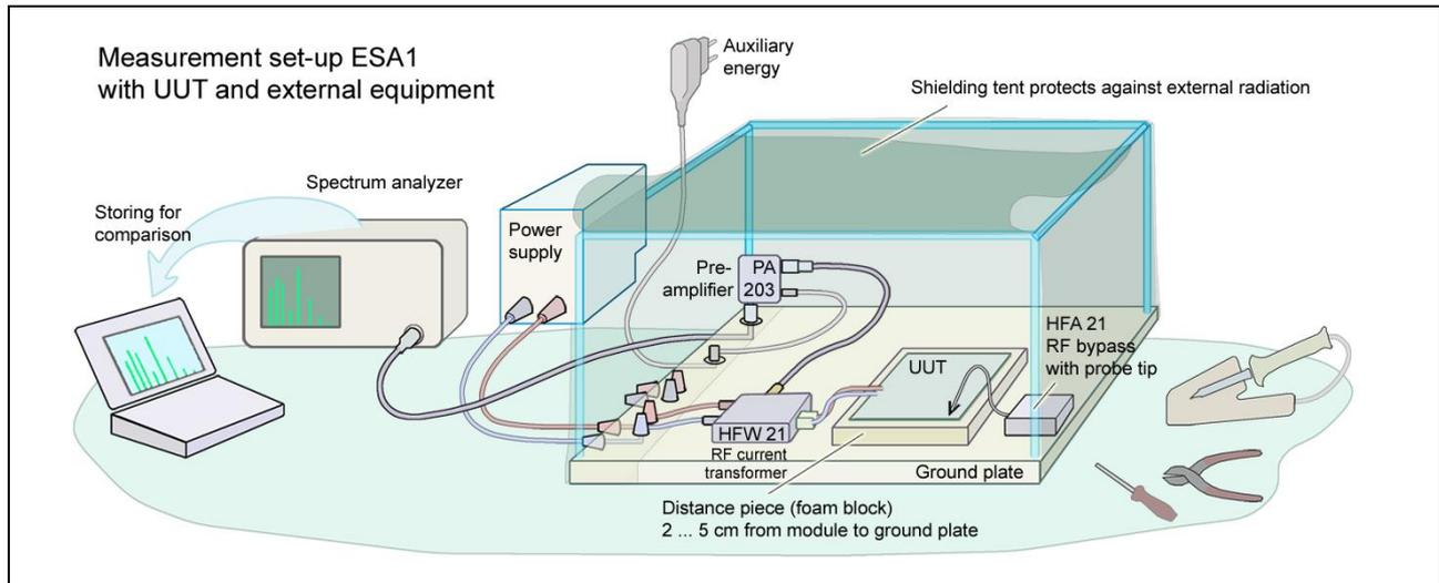
**Figure 15** Measurement set-up ESA1 (schematic)
