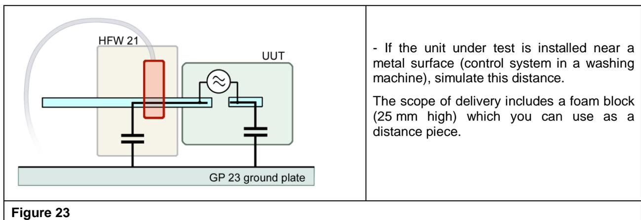
The capacitance between the unit under test and ground plate is determined by the size and distance of the unit under test. The RF current flows through this parasitic capacitance. This may be caused by electric fields on the surface of the unit under test which are generated by large surface clocked bus systems.
