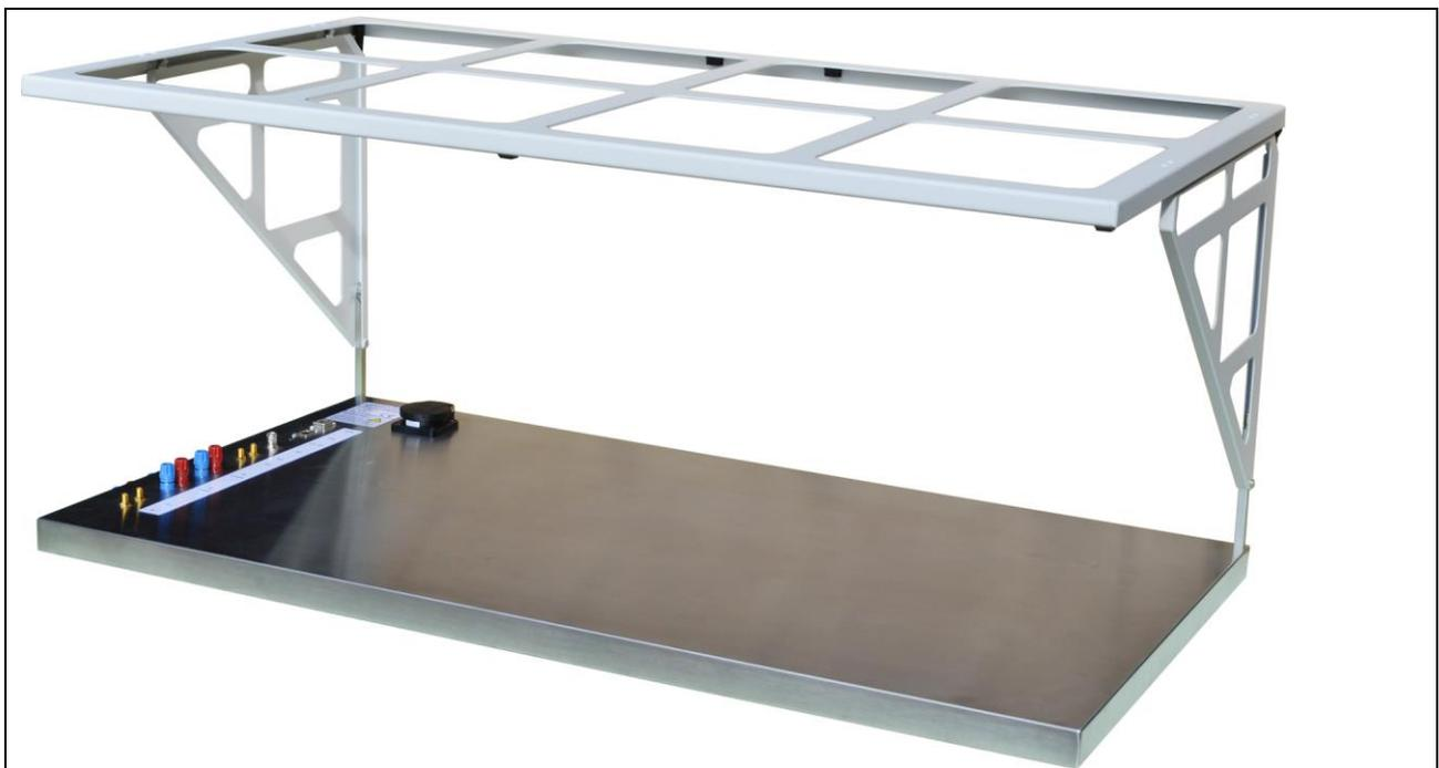
**Figure 5** ZG 23-1 set up on the GP 23 ground plate
