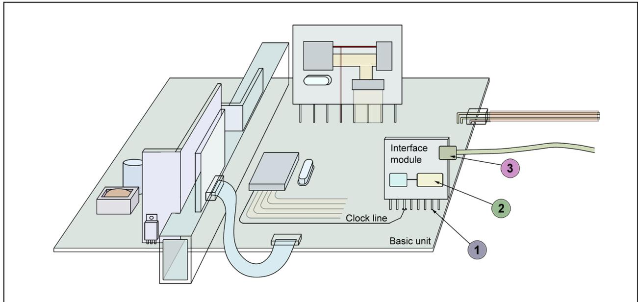
**Figure 27** RF sources on the interface module
