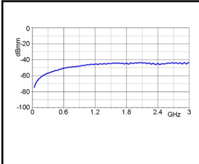
**RF-E 05** With this probe you are able to register selectively electrical fields on layouts and component area of flat units. The breadth of the field electrode is about 1 mm. Therefore you can locate electrical fields very accurately. These electrical fields are caused by clocked lines, IC pins and small components.
